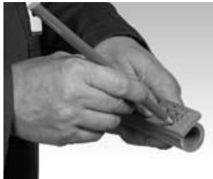
Marking of the welding depth
