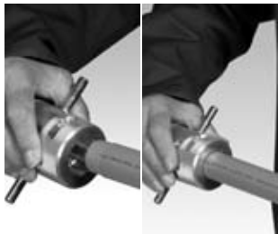
Peeling off the aluminium-PP-composite-layer respectively oxygen barrier layer (Necessary only for stabi-composite pipes, climatherm OT pipe and pipes with UV protection layer!)
