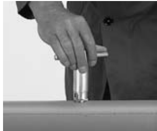
Removal of the aluminium layer from the stabi composite pipe.
