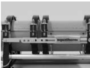
Join the pipes, cool down under pressure
